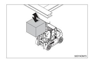
A Watch overhead clearance: Moving into overhead structures can tip a truck over, or spill a load.
