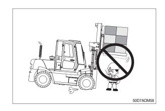
A Never use wire rope to lift a load.
