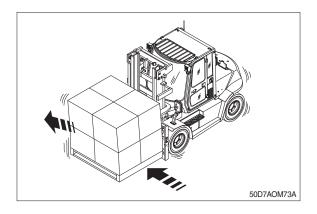
Never move the load to push or pull of it by the side shift.
